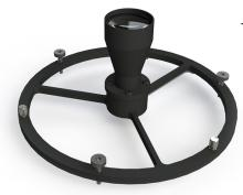
The fiber-coupled receiver mounts within the center shadow of the transmitted beam and collects a second data set coincident with the normal MPL data acquisition. This second channel has a larger field of view and is able to resolve backscattered light from much lower than the MPL's native channel. Since the two receivers are collecting the same laser pulse, deriving the overlap calibration becomes a simple matter of comparing the two signals to obtain a scaler factor.
